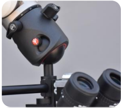
Ball joint for manipulation of laser head
