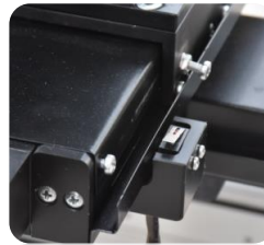
Limit switch for safe travel of the axis
