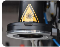
Laser protected ringlight for illumination of welding area
